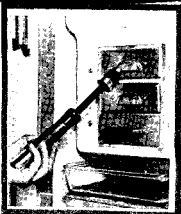
LOOSENS ICE TRAY. Tipped with rubber, this tool is specially designed for use in prying out ice trays. Handle shoved forward against shank jars the tray loose
