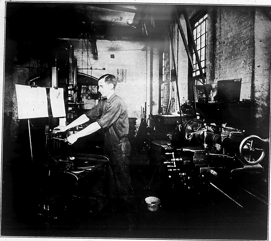
Fig. 13. Tool Stand, with the height gauge and packing piece racks and rack for holding drawing and instruction card for work in progress.
